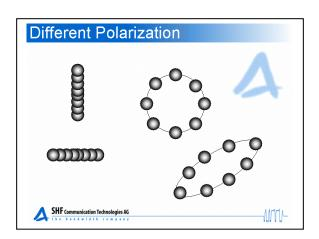
Linear Polarization is shown here: Note that the amplitude of Ex and Ey can vary, the polarization will stay linear.
