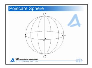
The state of polarization is described by the Stokes parameter:
