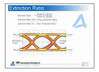
Lets go back to the example on page 3: The optical signal had an optical power of 100  $\mu$ W when a "0" was transmitted and an optical power of 1000  $\mu$ W when a "1" was transmitted, this translates to an extinction ratio of 10.
