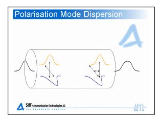
Due to birefringence different states of polarization travel with different speed, this causes pulse broadening.
