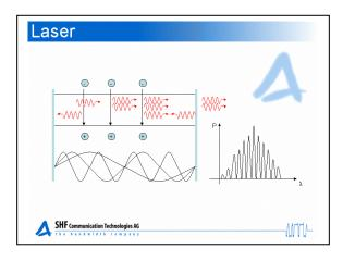
In a <u>D</u>istributed <u>Feedback</u> laser, distributed feedbacks (reflections) inside the resonator suppress all possible modes but one.
