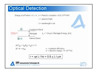
A photodetector generates a photocurrent according to the amount of incoming light and its responsivity. The photocurrent is converted into a voltage by a amplifier or a resistor.
