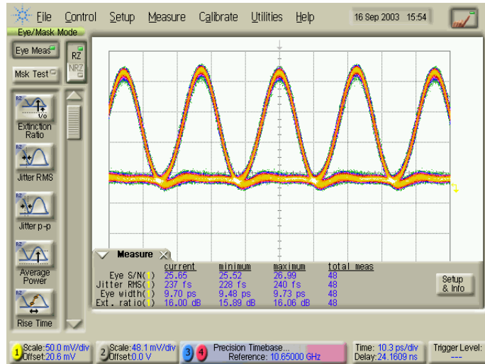
42.6 Gbps RZ optical output signal. S/N: 25.7; RMS Jitter: 237 fs
