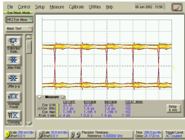
Output signal amplitude: 1.19 V
