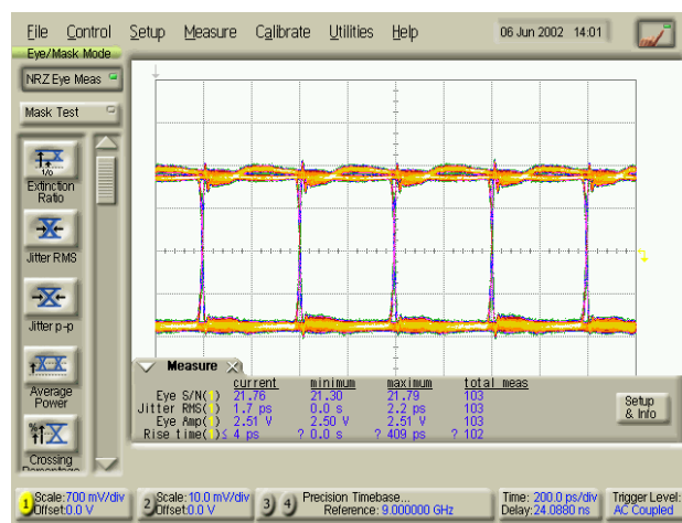
Output signal amplitude: 2.51 V
