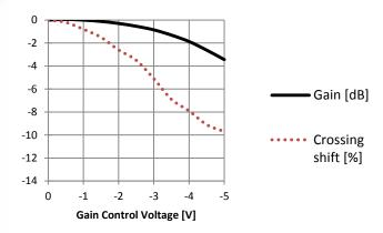
The crossing can be adjusted by applying a voltage of -5 to +5 V. If this pin is left open a crossing of approximately 50 % is achieved. The range depends on the input voltage. Typical characteristics are shown in the following diagram for input voltages of 0.4, 0.8 and 1.2 V with 50% crossing.
