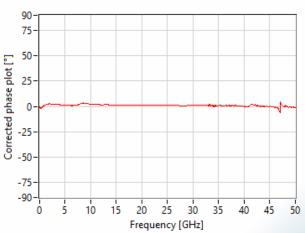
Aperture of group delay measurement: 160 MHz S21 phase measurement has been compensated by propagation delay to visualize phase linearity.
