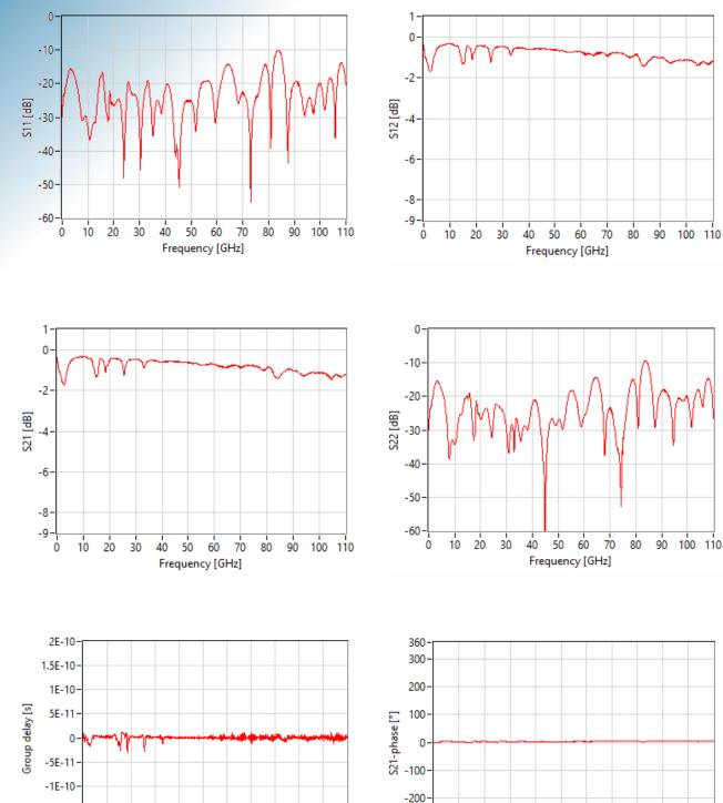
Aperture of group delay measurement: 160 MHz S21 phase measurement has been compensated by propagation delay to visualize phase linearity.
