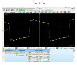
2.00 GHz output signal @ Clk DIV1 Out  $f_{out} = f_{in} \ /(2 \times N1), \ N1 = 1$
