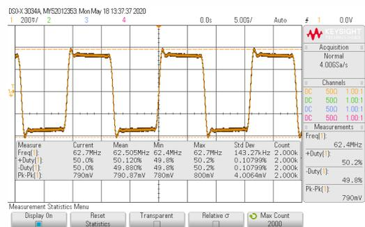
**62.5 MHz output signal @ Clk DIV<sub>2</sub> Out**
