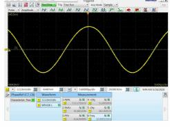
32.0 GHz output signal @ Clk /2 Out  $f_{out} = f_{in} \ /2$
