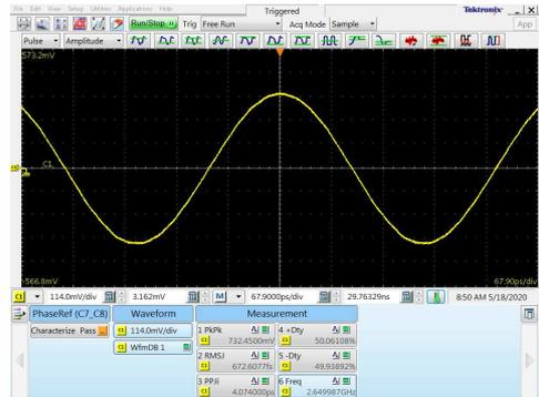
2.65 GHz output signal @ Clk DIV<sub>2</sub> Out
