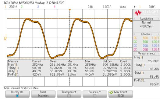
**251.97 MHz output signal @ Clk DIV<sub>2</sub> Out**
