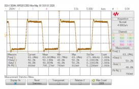
62.99 MHz output signal @ Clk DIV<sub>2</sub> Out
