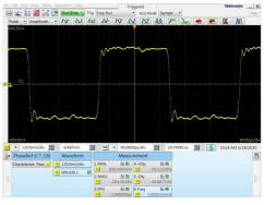
2.0 GHz output signal @ Clk /2 Out  $f_{out} = f_{in} /2$
