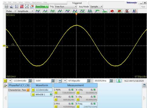
2.67 GHz output signal @ Clk DIV<sub>2</sub> Out
