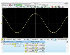
2.00 GHz output signal @ Clk DIV<sub>2</sub> Out  $f_{out} = f_{in} / (2 \times N_1 \times N_2), N_1 = 1, N_2 = 1$
