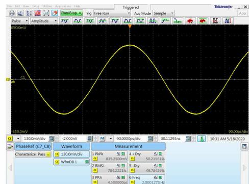
2.00 GHz output signal @ Clk DIV<sub>2</sub> Out
