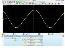
26.5 GHz output signal @ Clk /2 Out  $f_{out} = f_{in} \ /2$
