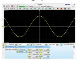
2.67 GHz output signal @ Clk DIV<sub>2</sub> Out  $f_{out} = f_{in} / (2 \times N_1 \times N_2), N_1 = 6, N_2 = 2$
