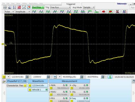
2.00 GHz output signal @ Clk DIV<sub>1</sub> Out
