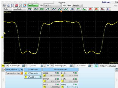
5.33 GHz output signal @ Clk DIV<sub>1</sub> Out
