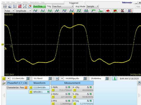
5.30 GHz output signal @ Clk DIV<sub>1</sub> Out
