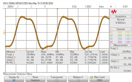
**250 MHz output signal @ Clk DIV<sub>2</sub> Out**
