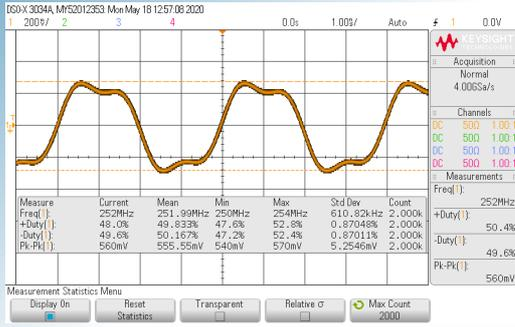
**251.97 MHz output signal @ Clk DIV<sub>1</sub> Out**
