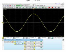
2.65 GHz output signal @ Clk DIV<sub>2</sub> Out  $f_{out} = f_{in} / (2 \times N_1 \times N_2), N_1 = 5, N_2 = 2$
