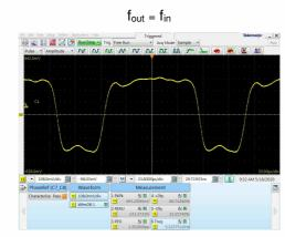
5.33 GHz output signal @ Clk DIV1 Out  $f_{out} = f_{in} \ /(2{\times}N1), \ N1{=}6$
