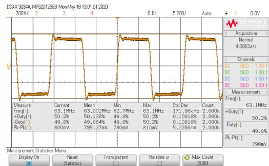
**62.99 MHz output signal @ Clk DIV<sub>2</sub> Out**
