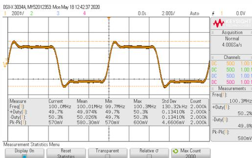
100 MHz output signal @ Clk DIV<sub>1</sub> Out
