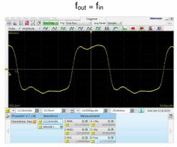
5.30 GHz output signal @ Clk DIV1 Out  $f_{out} = f_{in} \ /(2{\times}N1), \ N1{=}5$
