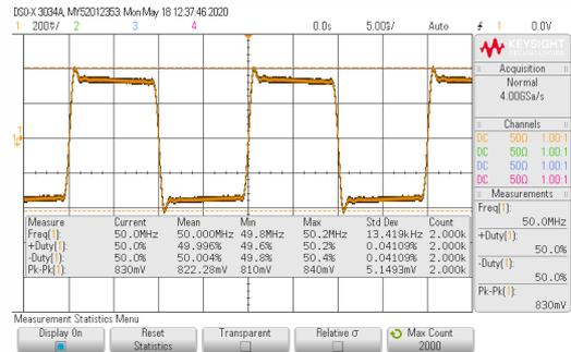
50 MHz output signal @ Clk DIV<sub>2</sub> Out
