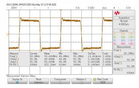
50 MHz output signal @ Clk DIV<sub>2</sub> Out
