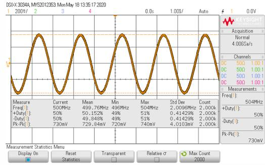
**500 MHz output signal @ Clk DIV<sub>2</sub> Out**
