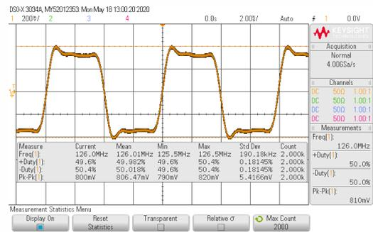
**125.98 MHz output signal @ Clk DIV<sub>2</sub> Out**
