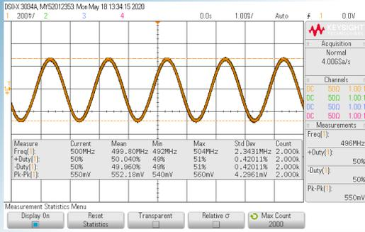
**500 MHz output signal @ Clk DIV<sub>1</sub> Out**
