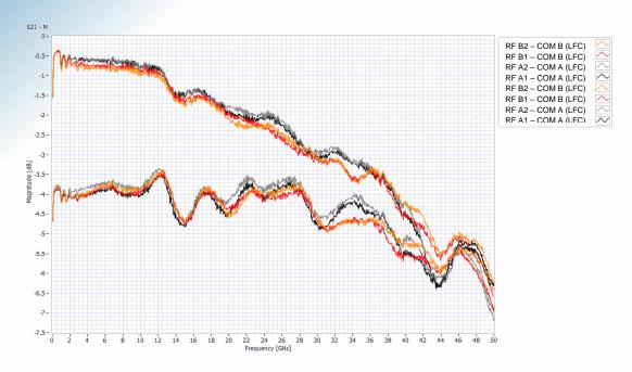
Insertion Loss - LFC compared to "no Option"
