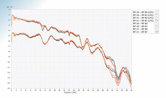
Insertion Loss - LFC compared to "no Option"
