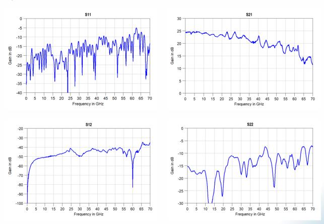
Fig.2: S-Parameter measurements @  $P_{in} = -30 \text{ dBm}$
