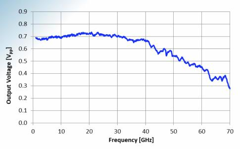
Fig.1: Output voltage @  $V_{in} = 200 \text{ mV}_{pp}$
