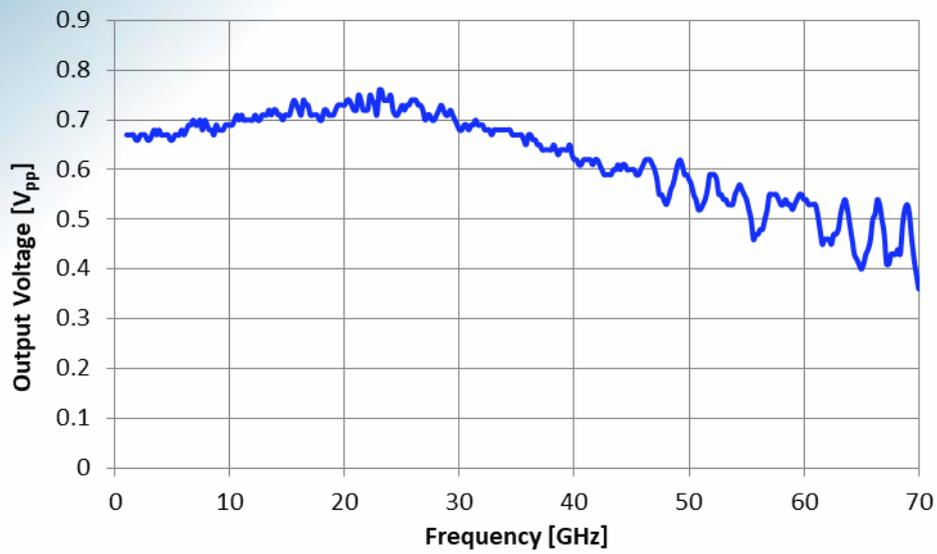
Fig.1: Output voltage @  $P_{in} = 200 \text{ mV}_{pp}$
