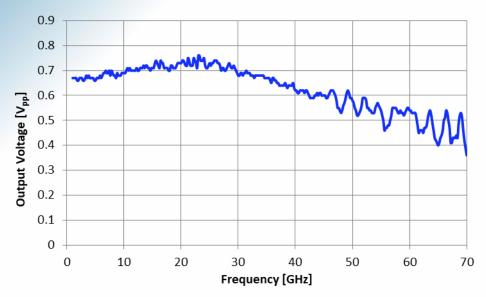
Fig.1: Output voltage @  $P_{in} = 200 \text{ mV}_{pp}$
