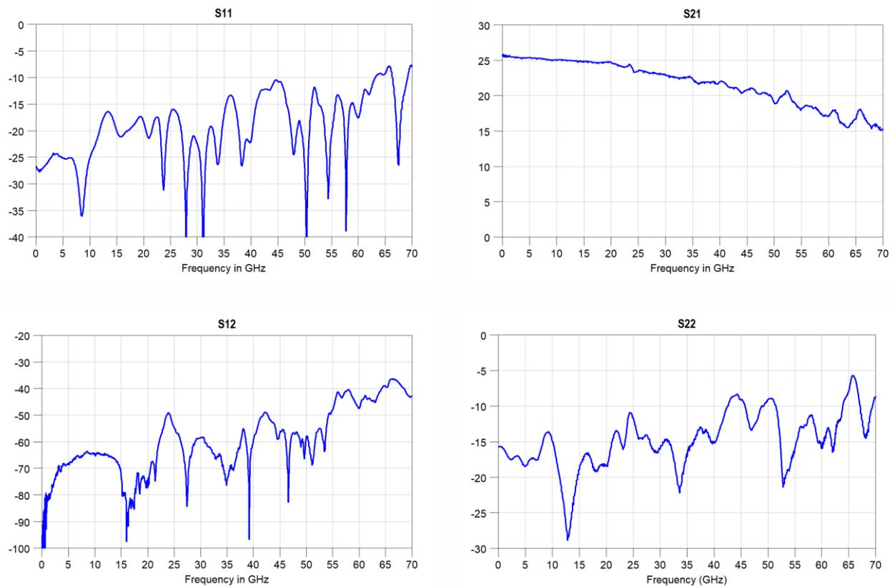
Fig.2: S-Parameter measurements @  $P_{in} = -30 \text{ dBm}$
