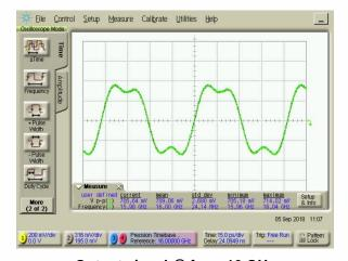
Output signal @ f<sub>out</sub> = 16 GHz
