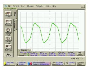
Output signal @ f<sub>out</sub> = 21.5 GHz
