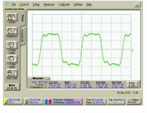
Output signal @ f<sub>out</sub> = 8 GHz
