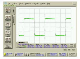
Output signal @ f<sub>out</sub> = 0.5 GHz
