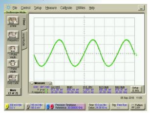
Output signal @ f<sub>out</sub> = 30 GHz
