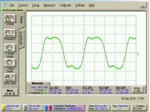
Output signal @ f<sub>out</sub> = 12.5 GHz
