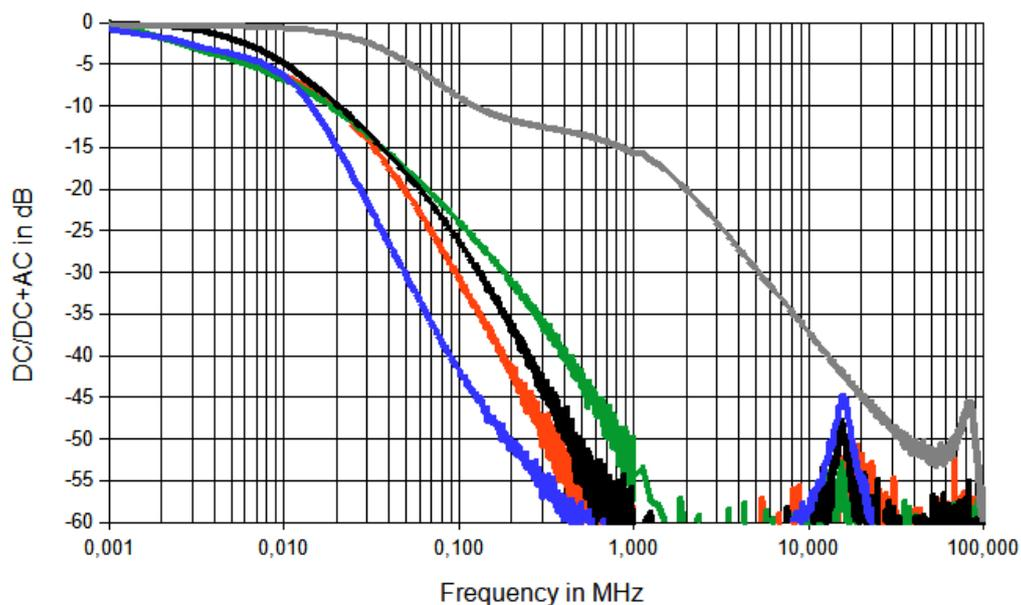
Note: The isolation DC/AC is better at low frequencies by the effect of the coupling capacitor in this path.
