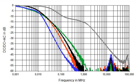
Note: The isolation DC/AC is better at low frequencys by the effect of the coupling capacitor in this path.
