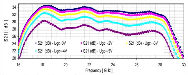
$S_{21}$  measured at different gain control voltages. Power in = -2dBm
