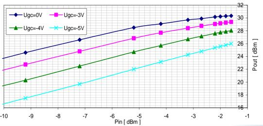
Output power vs. input power at different gain control voltages. Measured at 20GHz
