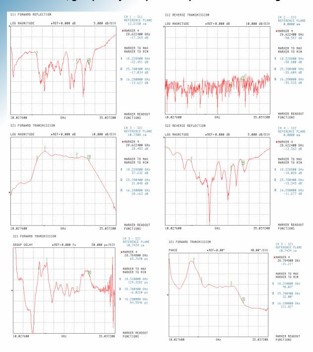
Aperture of group delay measurement: 81 MHz
