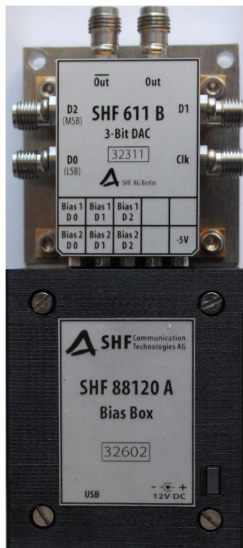
Fig. 1: "SHF 611 B + Bias Box"-Assembly
