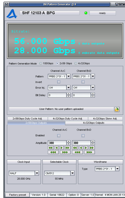
Controlling the dual 56 Gbps outputs
