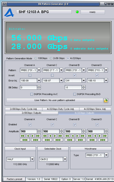
Controlling the quad 32 Gbps outputs
