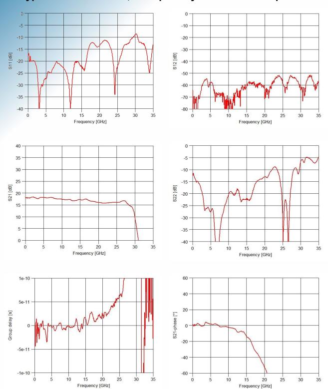
Aperture of group delay measurement: 100 MHz
