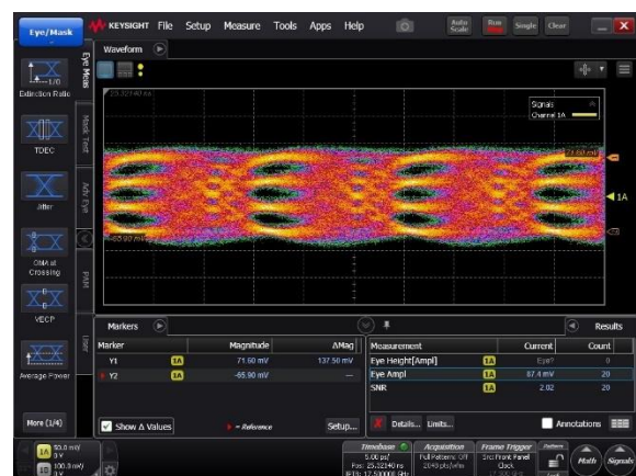
PAM4 @ 70 GBaud with equalization
