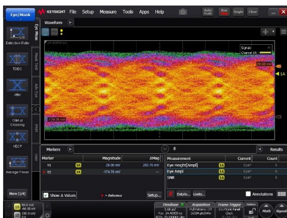
PAM4 @ 80 GBaud without equalization
