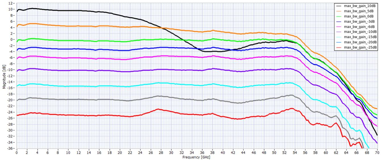
Frequency responses for a 3, 6, 9 and 12 dB slope @ 35 GHz
