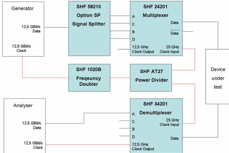
If your device under test has several meters of fiber, you will need a clock recovery such as the SHF 41210B Option CR or SHF 11120C at the demultiplexer, using the same clock for multiplexer and demultiplexer will not work due to the jitter and phase walk off caused by the fiber.
