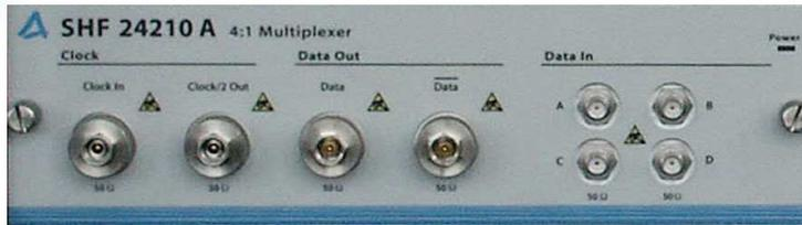
The most important instrument to upgrade a pattern generator to 50 Gbps is the multiplexer **SHF 24210A**.
