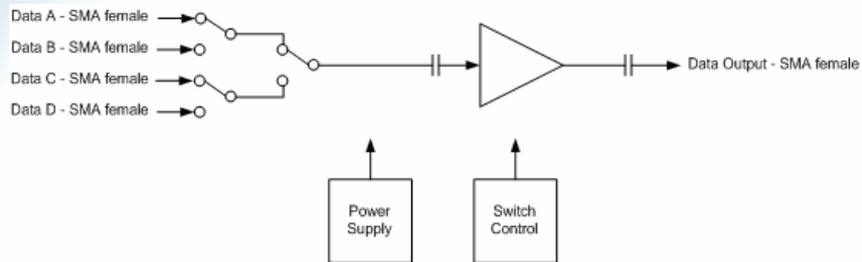
The module SHF58210A can be equipped with both or with only one of the two functional blocks (Signal Splitter *SP* and Signal Selector *SE*). Extra flexibility and cost efficiency are the benefits for the customer.
