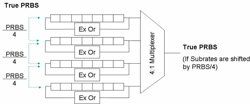
In the SHF 58210A Option SP signal splitter the delay to de-correlate the four sub-rates is done by cables – consequently (if the device is not used with PRBS  $2^7-1$  @ 4 x 9.953 Gbps) the output signal will not be true PRBS, it will be a Quasi PRBS sequence.
