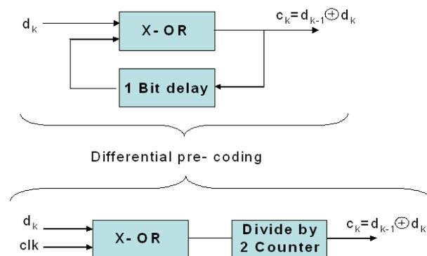
If you will be using your BERT system to generate and analyze optical DPSK or duobinary signals you might want to consider a 50 Gbps pattern generator: As DPSK and duobinary transmission requires precoding you would need a precoder if your test signal would be QPRBS.
