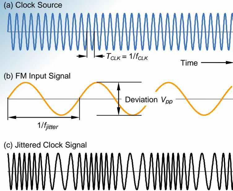
**Figure 2: Generation of a jittered clock signal by sinusoidal frequency modulation.**
