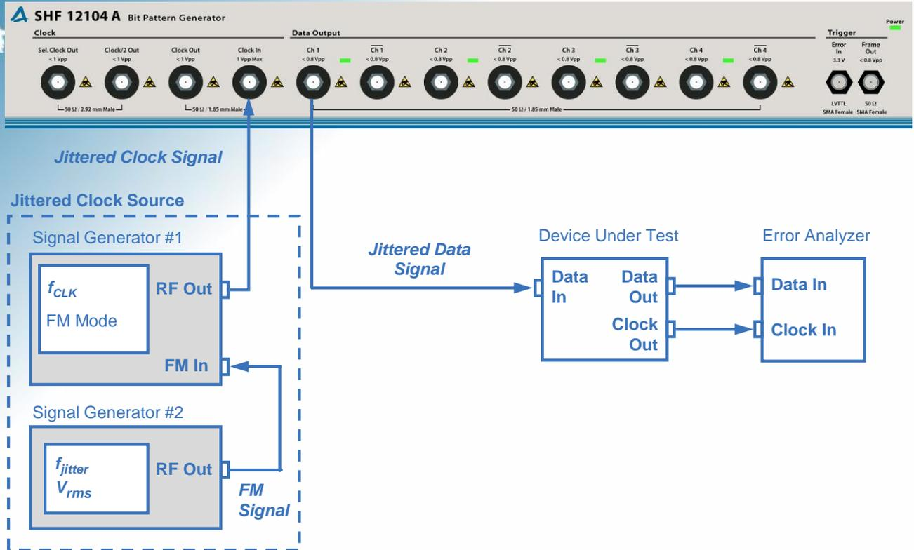
Figure 3: Jitter tolerance setup using the SHF 12104 A BPG.
