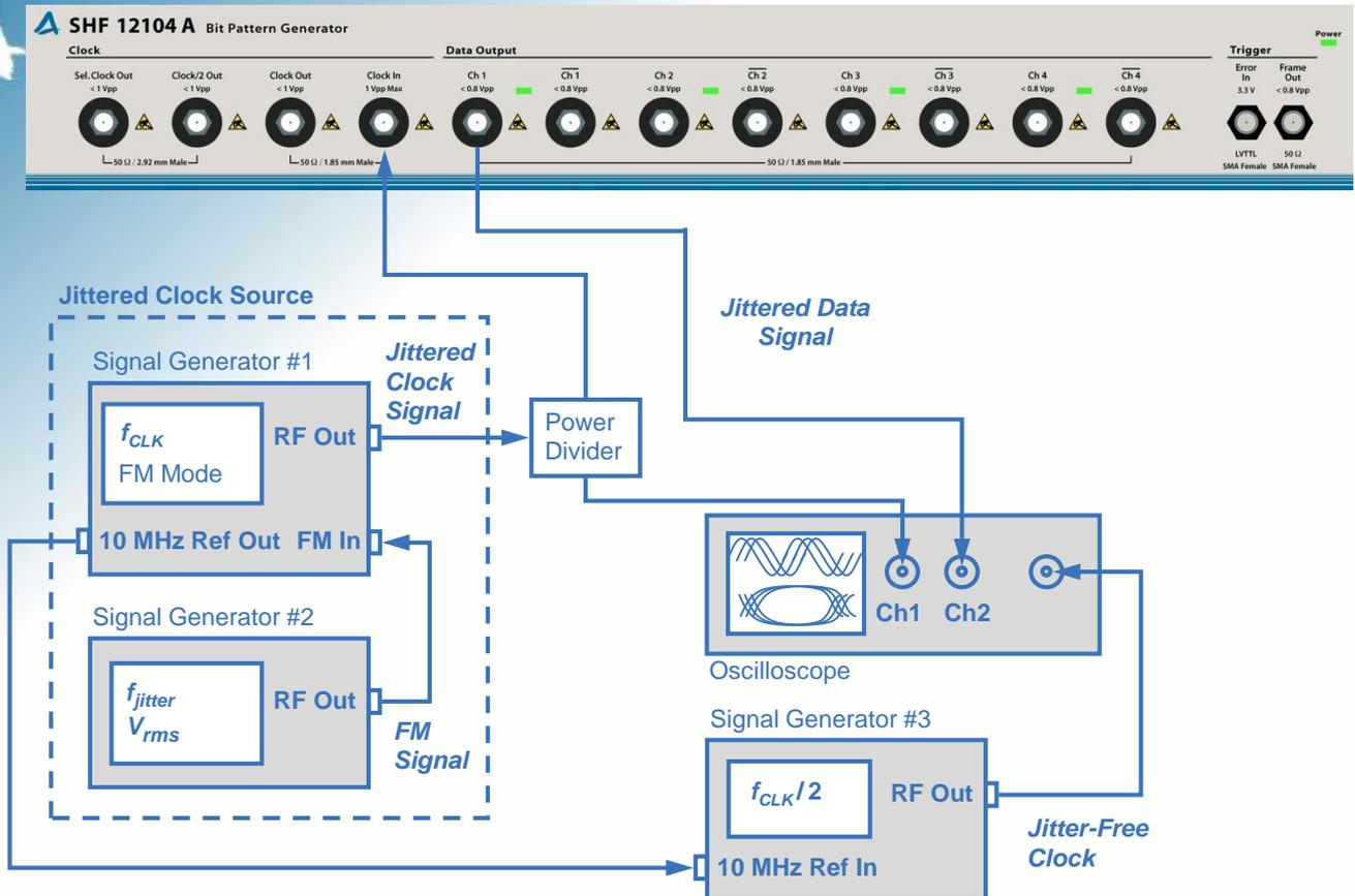
Figure 4: Jitter calibration and verification setup for the time-domain analysis of jittered signals.
