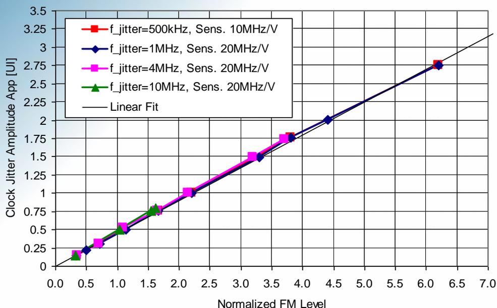
**Figure 8: Jitter amplitude imposed on a 28 GHz clock signal versus the normalized FM level obtained using the presented jitter injection setup for a range of jitter frequencies.**
