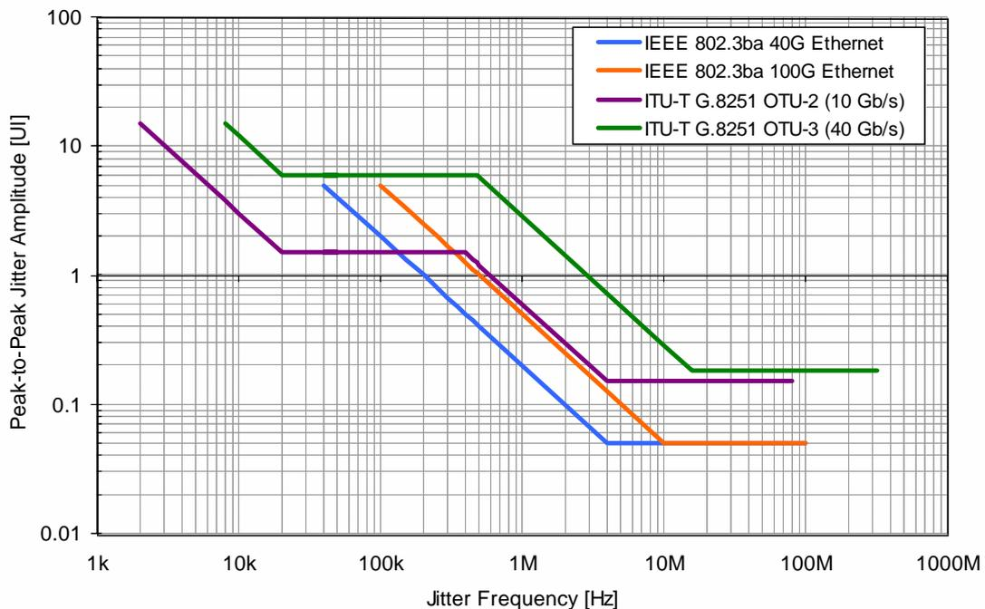
Figure 1: Sinusoidal jitter tolerance masks as defined in relevant communication industry standards [1], [2].
