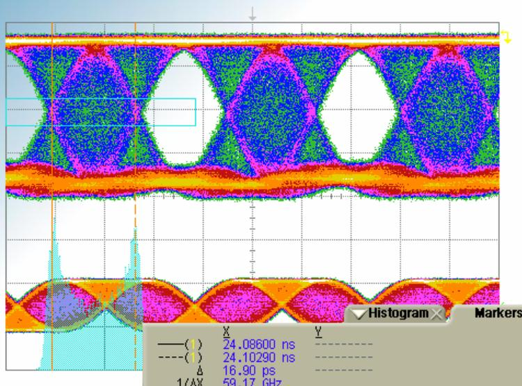
**Figure 5: Jittered clock eye diagram with 0.47 UI jitter amplitude at 28 GHz clock frequency (bottom) and jittered PRBS data eye at 28 Gbit/s with the same amount of jitter transferred from the clock (top).**
