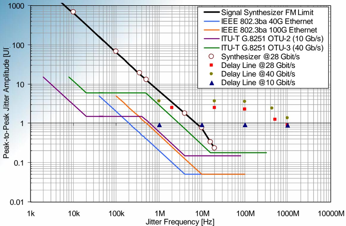
**Figure 9: Maximum achievable sinusoidal jitter amplitude versus jitter frequency using the SHF 12103 A or SHF 12104 A BPG.**
