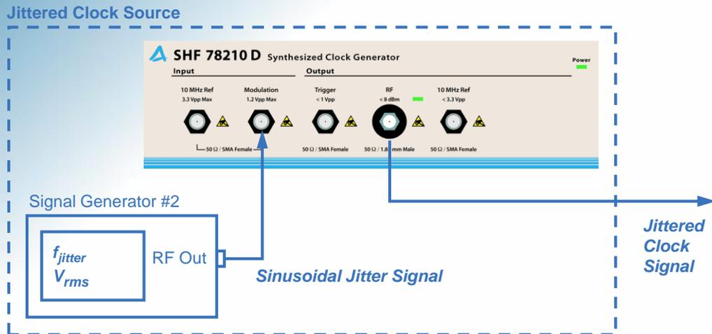
Figure 10: Jittered clock source using SHF 78210 D.
