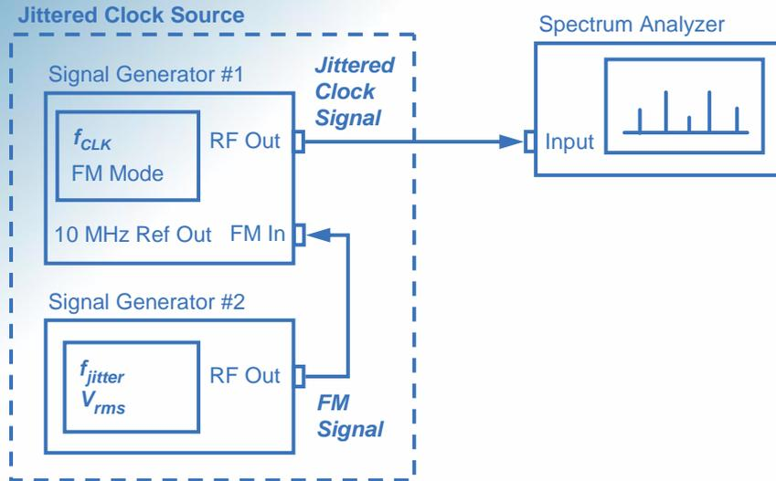
Figure 6: Jitter calibration and verification setup using a spectrum analyzer.
