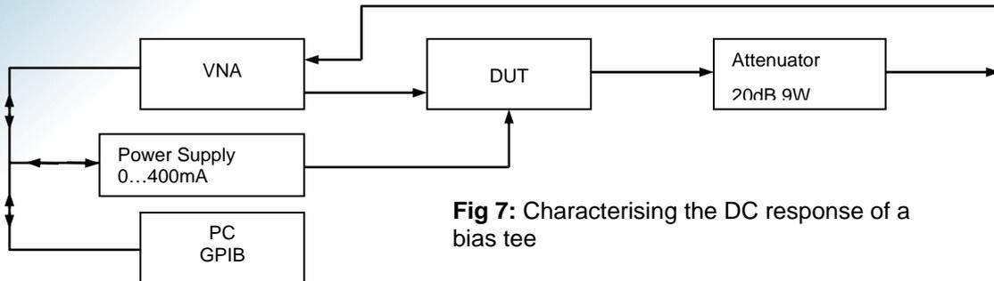
**Fig 7:** Characterising the DC response of a bias tee
