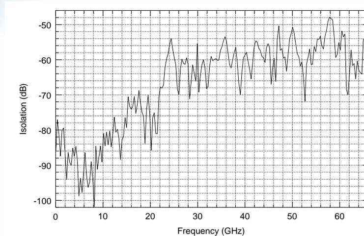
**Fig 9** Isolation measured between the bias port and HF-in port.
